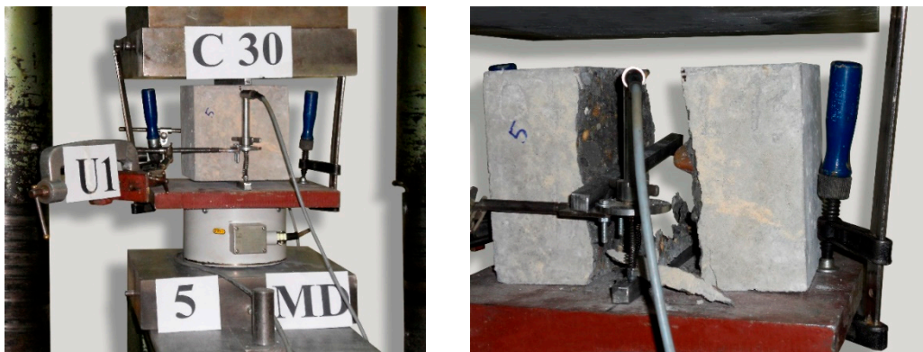
Figure 4. Experimental setup for induced tensile load capacity in a concrete sample.
